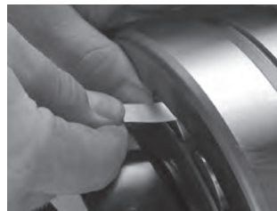
Fig. E-3. Measure RIC before installation.
