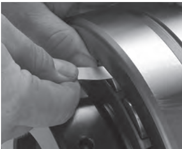
Fig. E-7. Measure RIC before installation.
